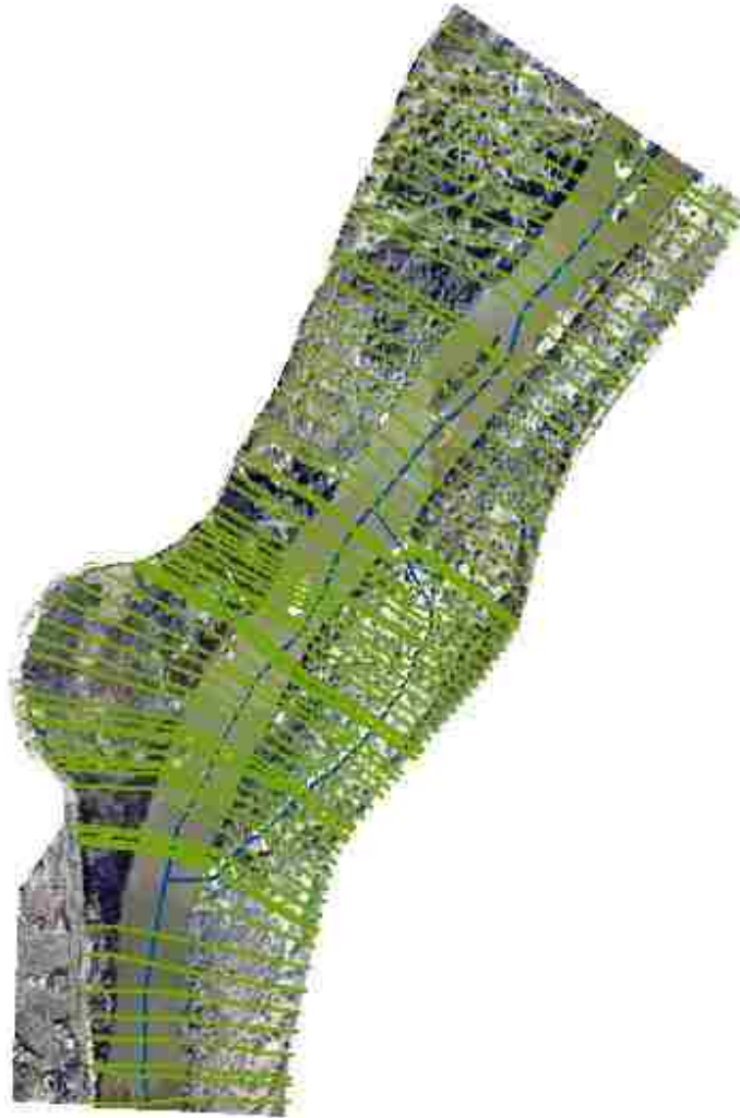
Figure 3-1: Plan View of First HEC-RAS Model Geometry
